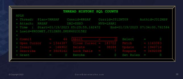
All of the highlighted Red displayed statistics need to be further investigated. The most important highlighted consideration is the ABORT = 2 situation. Given that the statistics show the process has Inserted, Deleted and Updated so many rows it could be a rollback situation or data integrity problem.
