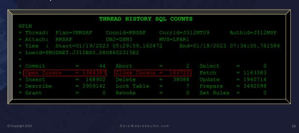
In a DB2 Java application, the DB2 SQL OPEN and CLOSE cursor counts should be the same to ensure optimal performance and efficient use of system resources. When a cursor is opened, resources such as locks and buffers are allocated to the cursor. These resources are only released when the cursor is closed.
